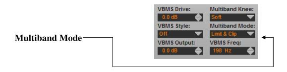
The Multiband Mode control is present <u>only</u> on the AP1000 product and selects one of four different operating modes for the 31 band limiter and its associated 31 band distortion masked clipper.
