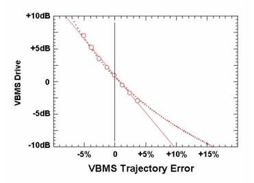
If it were possible, theoretically perfect behavior would be represented by the vertical line extending above the "0" on the horizontal axis.
