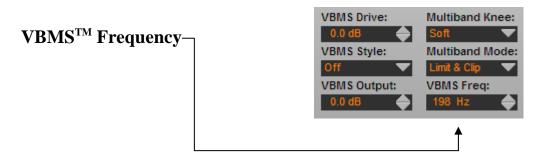
The VBMS<sup>TM</sup> Frequency is adjustable over the range of 60Hz to 300Hz with audio information that is present <u>below</u> the Frequency setting being processed by the algorithm.
